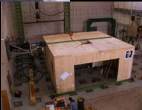
Pseudo- dynamic tests on one storey specimen
