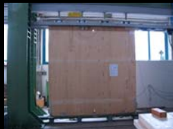
Pseudo- dynamic tests on one storey specimen
